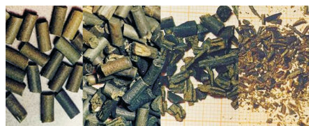
Fig. 2 Ageing of NC grains, leading to an increasing grain fracture during firing
